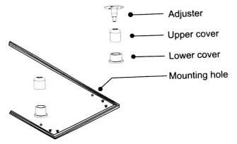
4、Adjust height of 4 strips to make the light parallel to the ceiling, and install LED driver, switch on the light.
